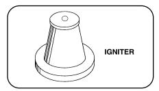
The cooktop uses electronic igniters to light the burners. Each burner has its own igniter that sparks when any burner is turned on. When the igniters are clicking (sparking), do not touch the burners. If a burner fails to ignite, see "Before Calling For Service," Page 28.
